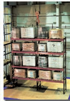
Base Isolated Storage Rack
