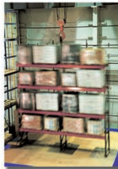
Base Isolated Storage Rack
