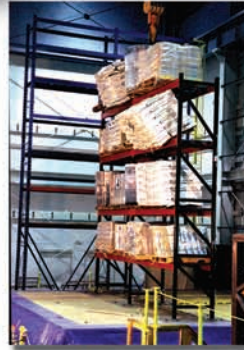
Fixed-Base Storage Rack (without Isolators)
