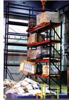
Fixed-Base Storage Rack (without Isolators)
