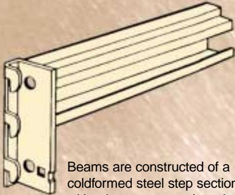
Beams are constructed of a coldformed steel step section with a heavy gauge, three lug hook connector welded to each end of the step section. The smooth face of beam enables easy labeling while minimizing exposed edges. The steps on the beams redesigned to accommodate plywood or particle board drop-in shelves of standard dimensions.
