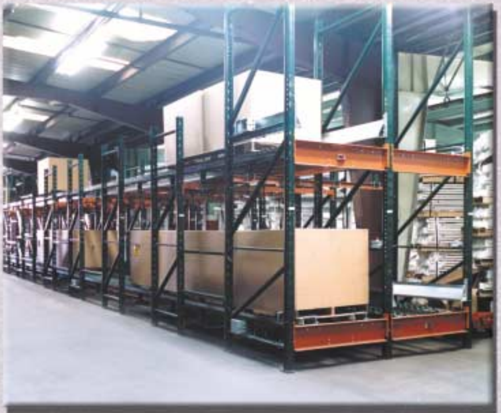
Pallet move through the system propelled by a series of motorized carts.
