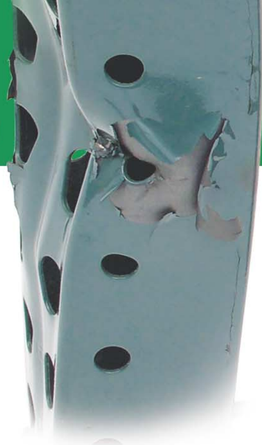
Guillotine Impact Testing best simulates the impact of a lift-truck fork.
