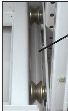
The "V" roller shelf guide mechanism
